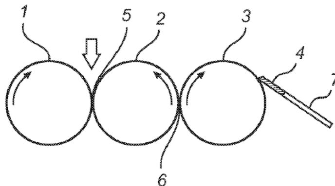
**Figure 1.** Schematic drawing of three-roll mill: (1) feed roll, (2) center roll, (3) discharge roll, (4) discharge blade, (5) first nip, (6) second nip, and (7) apron
