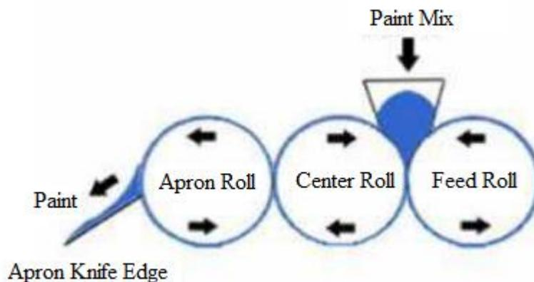
*Figure 1. The schematic drawing of three-roll mill*
